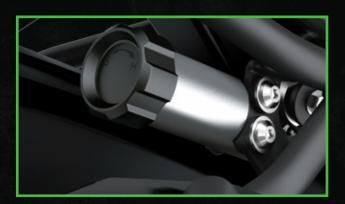
A remote preload adjuster means changes to suit tandem riding or luggage can be made quickly and easily by hand.
